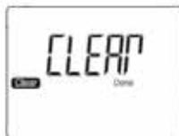
The function allows user to nullify the accumulated flow value. By selecting this menu (Clean), the accumulated flow will become zero. After press  $\text{Fun}$ , the screen will show "Setting...". Please do not interrupt until "Done" is displayed. The screen will then automatically return to the menu selection screen.
