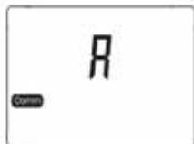
This function allows user to select single meter communication or communication network via RS485 (Modbus). After selecting this menu, the communication status is shown by the flashing letter at the center of the screen. **A** indicates single meter operation while **b** represents the Modbus networking status. Press  $\uparrow$  or  $\downarrow$  can change the current status to another. Then press  $\text{Fun}$  to confirm,
