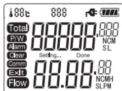
Interface includes *instant flow, accumulated flow; temperature and battery status; menu and other process data during setup.* See the graph at the left for details.
