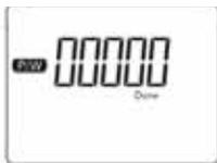
After the 5 digits are input completely, the interface will display "Setting...". Please do not interrupt until "Done" appears on the screen. The process usually takes 3 seconds, and then it will automatically return to the menu selection screen.
